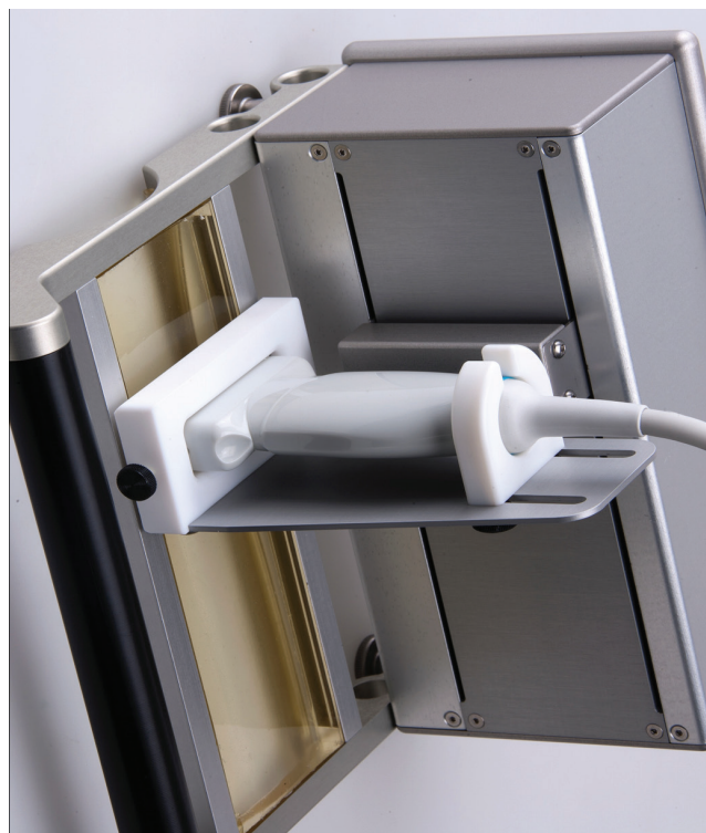
Figure 4: Ultrasound tissue characterization tracker frame with attached ultrasound probe and built in standoff. Image courtesy of Hans van Schie.
